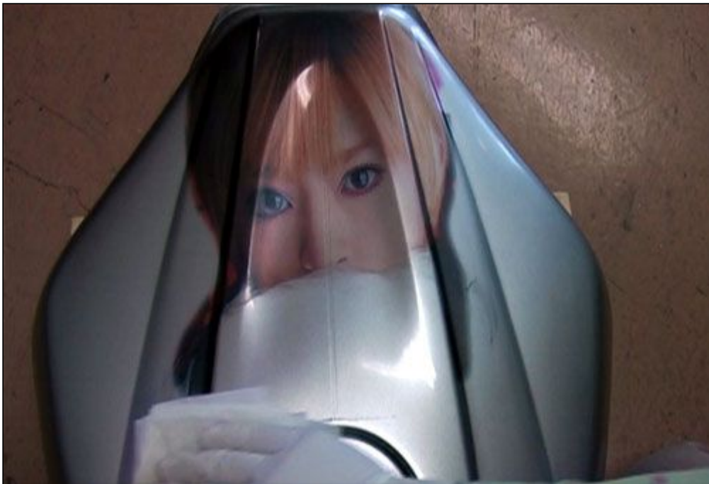
Printed image is erasable by acetone. You can reprint easily.
